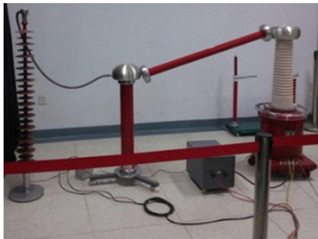
Fig. 22. The partial discharge instrument.
