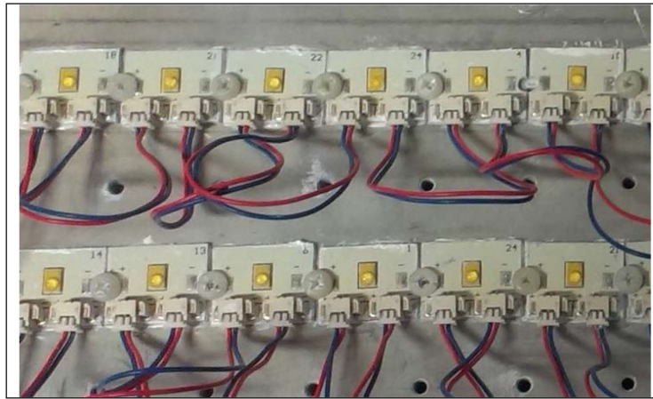
Fig. 1. Individual LEDs on metal core PCBs (MCPCB) mounted on aluminum heat sink.
