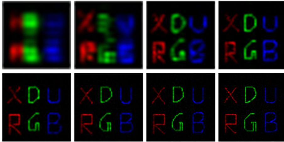
Fig. 7 Results of serial achromatic imaging through scattering media for different dimensions. The dimensions are 16 \times 16 , 20 \times 20 , 30 \times 30 , 40 \times 40 , 50 \times 50 , 60 \times 60 , 70 \times 70 , 80 \times 80 , respectively.
