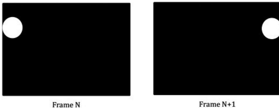
Fig. 19. The relative position of the LED in two successive frames.
