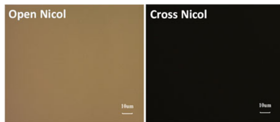
Fig. 1. Open Nicol (left) and Cross Nicol (right) images of 0.7 at.% Ho:Y 2 O 3 transparent ceramics on the microscopic scale.
