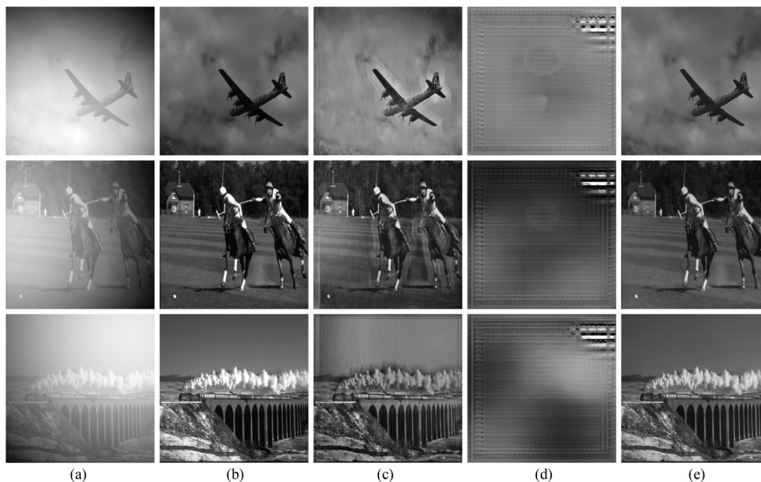
Fig. 8. Different CNN architectures in the denoising network produce results of different quality on the dataset 'b100'. The intensity of the optical noise is set to \delta = 0.01 . (a) Input images, (b) target images, (c) images corrected by ResCNN, (d) images corrected by EDCNN, and (e) images corrected by our method.
