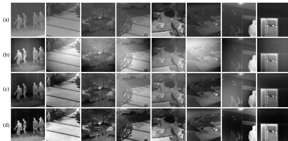
Fig. 4. Comparisons with Cao's method on the infrared dataset. The intensity of the optical noise is set to \delta = 0.002 . (a) the target images, (b) input images, (c) images corrected by Cao's method, and (d) images corrected by our method.
