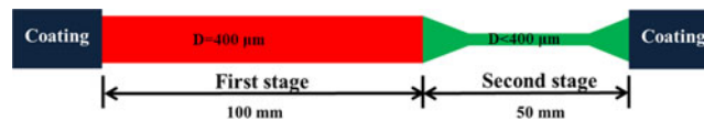
Fig. 1. Schematic illustration of the two-stage stripper. The first stage of the CLS was dealt with gradual chemical etching. The second stage was fabricated by reducing cladding diameter and roughing the fiber surface.
