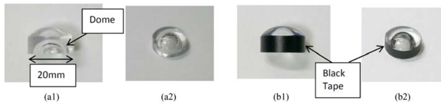
Fig. 10. (a1) and (a2) are respectively the front view and iso-angle view of the manufactured lens. (b1) and (b2) are the corresponding views of the same lens with a black tape applied to the vertical wall of the lens.
