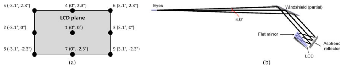
Fig. 4. (a) Nine fields (1 to 9), given by a horizontal angle followed by a vertical angle, and their corresponding positions on the LCD plane. (b) Side view of the light paths in the optimized HUD in LightTools software.
