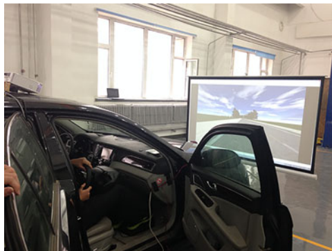
Fig. 10. Simulative automotive driving environment projected on a screen 2.5 m away from a subject.
