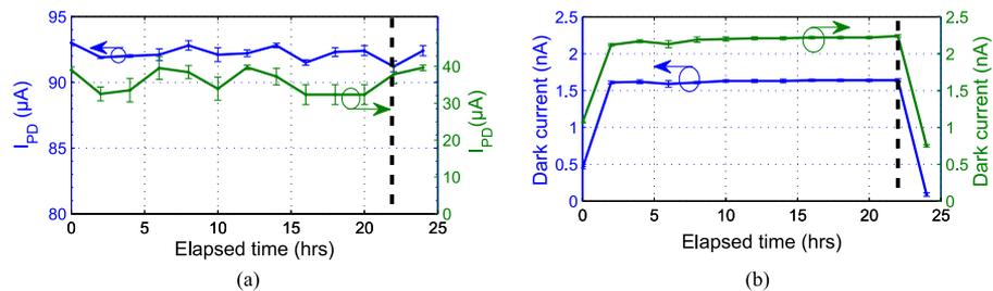
Fig. 10. Received current (a) and dark current (b) of the photodiode with the quartz ball lens as function of time (X-rays dose : 10.8 Mrad/hour).
