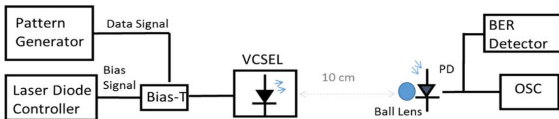
Fig. 1. OWC experimental setup at 2.5 Gb/s and 10 cm distance. OSC: Sampling oscilloscope; PD: PIN photodiode+TIA.
