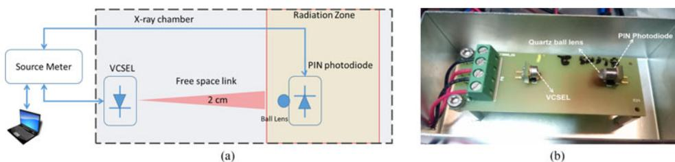
Fig. 7. (a): X-rays irradiation test setup; (b): PCB with the VCSEL and the photodiode with a ball lens.
