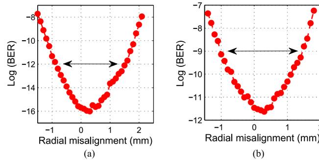
Fig. 4. Estimated BER vs. radial misalignment at 15 cm (a) and 20 cm (b) transmission distance.
