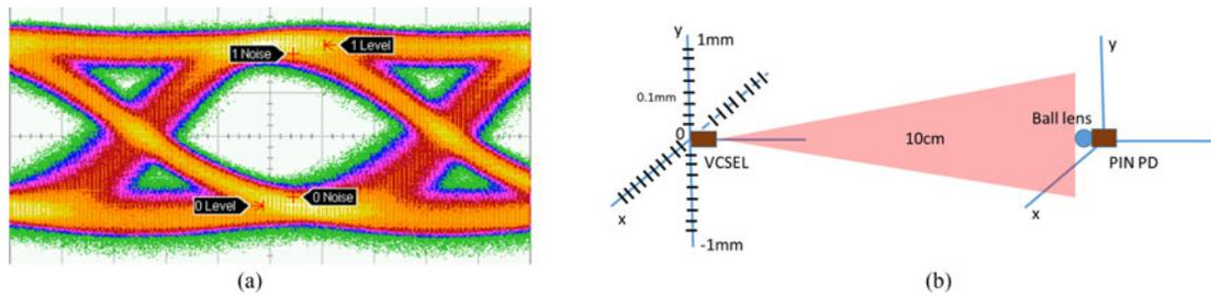
Fig. 2. (a): Eye diagram for the 2.5 Gb/s signal at 10 cm ; (b): tolerance measurement schematics.
