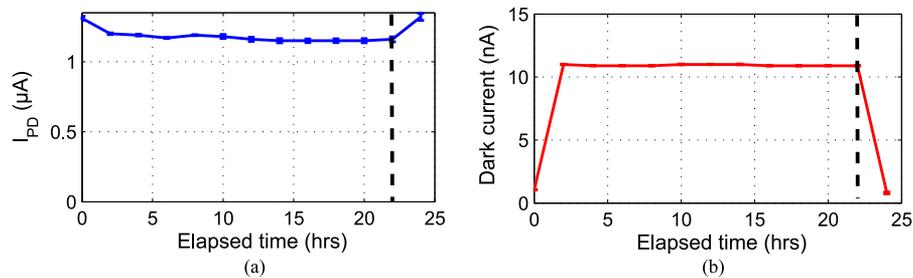
Fig. 9. (a): Received current at the photodiode as a function of time; (b): dark current of the photodiode at a reverse bias of 4 V as a function of time with 10.8 Mrad/hour dose. Bar line shows end of irradiation test.
