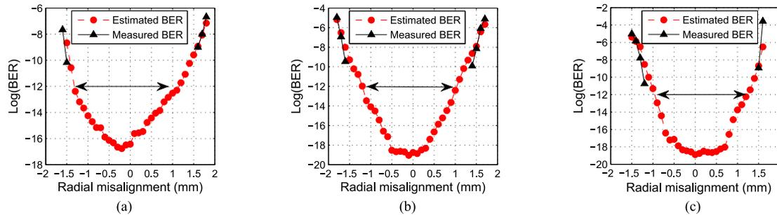
Fig. 3. Tolerance to misalignment: BER vs. radial misalignment for 3 mm (a), 4 mm (b), 5 mm (c) ball lens.
