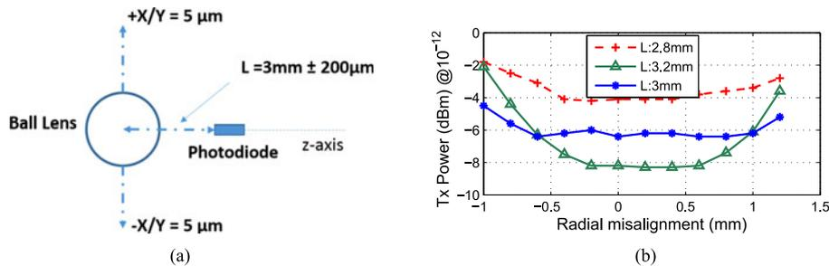
Fig. 5. (a): Scheme of packaging tolerance for the lens; (b): transmitted (Tx) power as a function of radial misalignment considering  $5 \mu\text{m}$  deviation on X/Y axis and for different values of L (z-axis).
