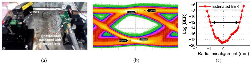
Fig. 6. (a): OWC experimental setup of 2.5 Gb/s; (b): eye diagram; (c): BER vs. misalignment.
