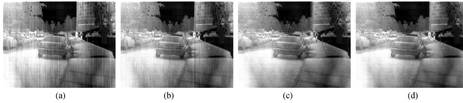
Fig. 6. Processing results using different spatial filtering schemes. (a) Raw image. (b) Correction result using a global model (height of N_v is set to the image height H ). (c) Correction result using a local model (height of window N_v is set to \frac{H}{16} ). (d) Correction result using our proposed spatially adaptive filtering scheme. The proposed method adaptively combines the advantages of global and local-based correction methods and achieves better performance on both eliminating column FPN and preserving image edges. Please zoom in to check details.
