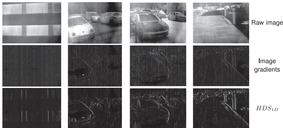
Fig. 5. Comparative results of image vertical structure extraction on raw infrared images which contain obvious column FPN. All images are normalized to 0-1 value range for visualization.
