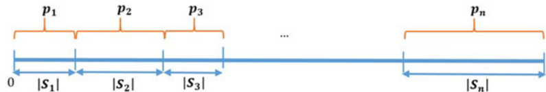
Fig. 4. Stochastic Universal Sampling technique for selecting the population members as crossover parents for next generation.
