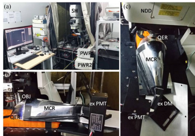
Fig. 5. The device, as illustrated in Fig. 1. (a) Overview, (b) side view, and (c) top view. SH:scan head of Nikon microscope; PWR 1&2:power supplies for ex PMT.
