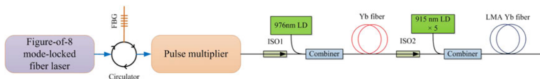
Fig. 1. Schematic diagram of the MOPA structured Yb fiber amplifier with multi-pulse operation.
