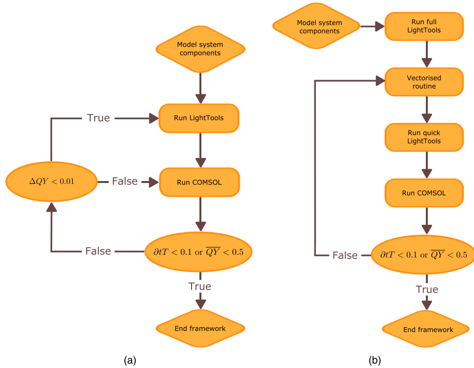
Fig. 4. Flowchart of the framework for the (a) general case and for the (b) vectorized approximation showing example values for the stopping conditions. Full LightTools refers to simulating the entire domain with LightTools, whereas quick LightTools refers to using the artificial source to bypass the phosphor simulation.
