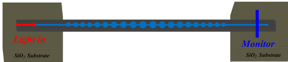
Fig. 4. Schematic diagram of the single 1-D PhC-SNC sensor obtained from 3D-FDTD optimization. The width of the silicon ( Si ) ridge waveguide and the slot are w_{nb} = 650 nm and w_{slot} = 50 nm, respectively. The periodicity of the holes is a = 559 nm, and the hole radius is parabolically tapered from r_{center} = 235 nm in the center to r_{end} = 203 nm on both sides with the number of gratings chosen to be i_{max} = 10 . The thickness of the silicon ridge waveguide is h = 220 nm for the entire device, which is symmetric with respect to its center. n_{si} = 3.46 .
