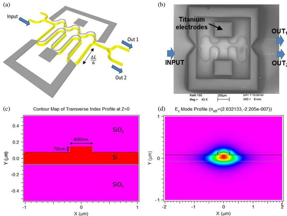
Fig. 1. (a) 3-D schematic of the a-MZI switching structure, where  $\Delta L$  is the length difference between the MZI arms, (b) SEM image of fabricated device, (c) cross section of the rib waveguide and refractive index distribution, and (d) fundamental transverse electric (TE) mode of the rib waveguide.
