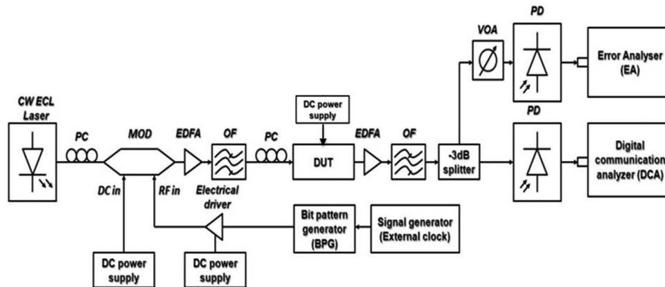
Fig. 6. Experimental set-up.
