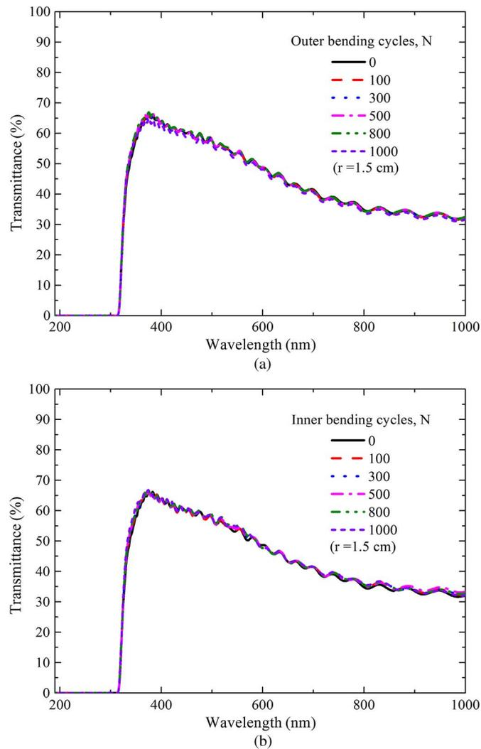
Fig. 5. Transparency of the stack PET/MoO<sub>3</sub>/Ag/MoO<sub>3</sub> as a function of the number of (a) outer or (b) inner bending cycles.
