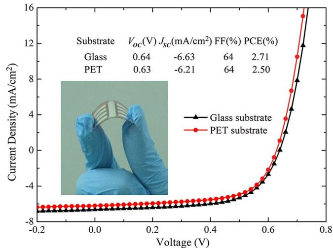
Fig. 2.  $J$ - $V$  characteristics for ITO-free OSCs fabricated on PET or glass substrates under 1 sun AM 1.5G simulated illumination. For comparison, the corresponding photovoltaic parameters have been shown here as an inset. Meanwhile, a photograph of a bent flexible ITO-free device is also shown the inset.
