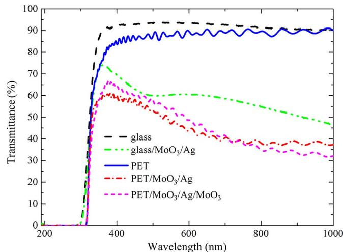
Fig. 3. Wavelength-dependent transmittance spectra of PET, glass, glass/MoO<sub>3</sub> (2 nm)/Ag (9 nm), PET/MoO<sub>3</sub> (2 nm)/Ag (9 nm), and PET/MoO<sub>3</sub> (2 nm)/Ag (9 nm)/MoO<sub>3</sub> (10 nm).
