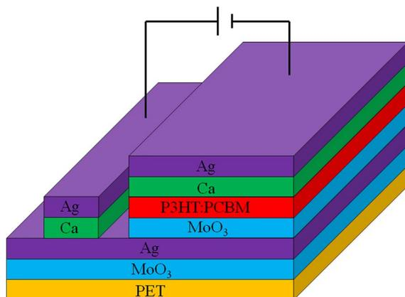
Fig. 1. Device geometry of ITO-free OSCs fabricated on PET substrates.
