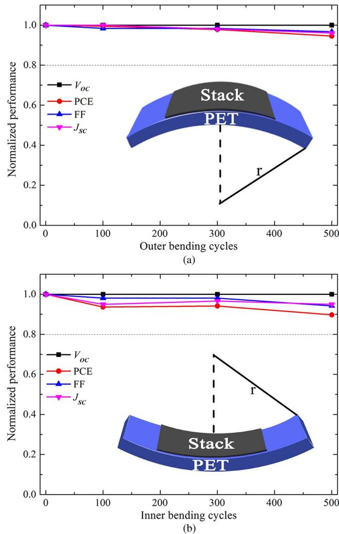
Fig. 4. Normalized photovoltaic performance parameters of flexible ITO-free OSCs as a function of the number of (a) outer or (b) inner bending cycles. (a) (Inset) Schematic drawing of outer bending configuration.  $r$  in the inset represents the bending radius. (b) (Inset) Schematic drawing of inner bending configuration.
