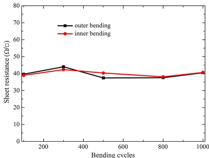
Fig. 6. Sheet resistance of the stack PET/MoO<sub>3</sub>/Ag/MoO<sub>3</sub> as a function of the number of outer or inner bending cycles.
