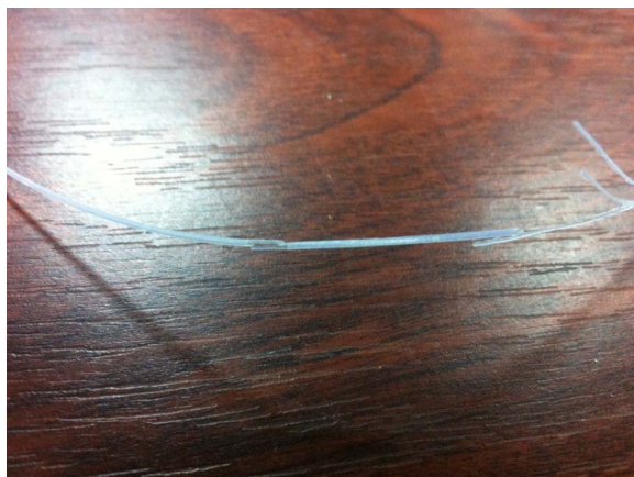
Fig. 10. The degradation of the LPG connecting fiber jacket.
