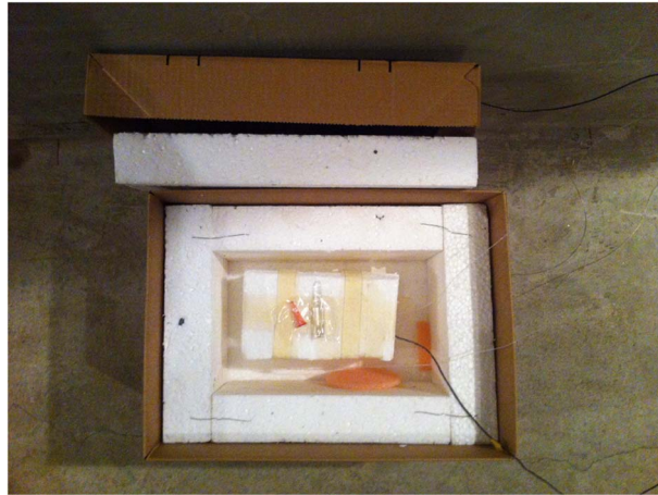
Fig. 5. The insulating box carrying the LPG during gamma irradiation.
