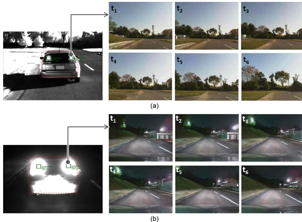
Fig. 16. Reception results (extracted per approximately 1 s) of consecutive front-view images. (a) Under the daytime lighting condition. (b) Under the nighttime lighting condition.
