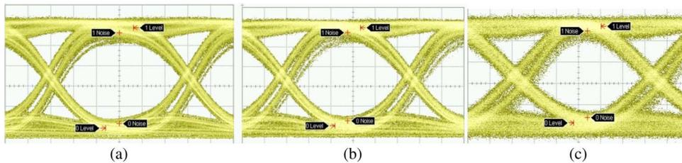
Fig. 6. Measured eye diagram at (a) 2.5 Gbps back-to-back. (b) 2.5 Gbps after 20 km SMF transmission. (c) 2.5 Gbps after 50 km SMF transmission.
