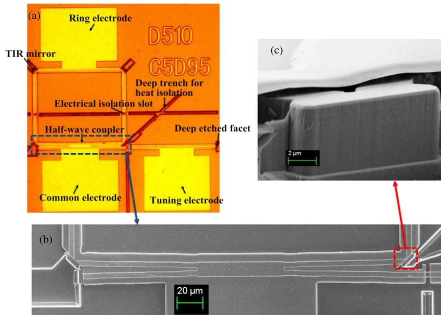
Fig. 1. (a) Optical microscope image of the half-wave coupled rectangular ring-FP laser; (b) SEM picture of the half-wave coupler; and (c) SEM picture of the etched mirror.
