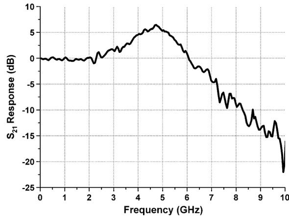
Fig. 5. Small signal frequency response of the laser. The modulation signal is applied on the common electrode.
