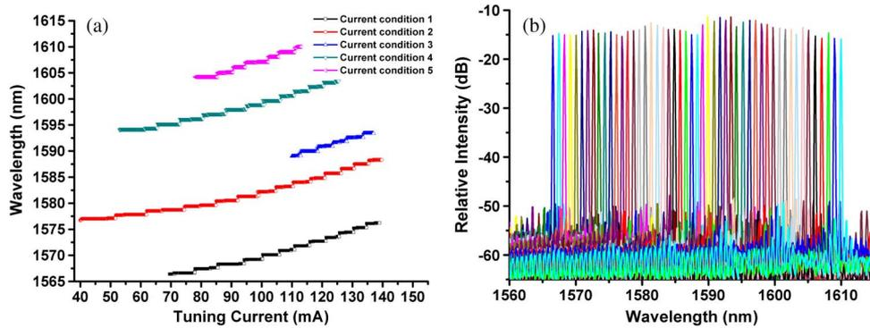
Fig. 4. (a) Measured five single-electrode-tuning curves under different injection currents on the common electrode and the ring electrode and (b) the corresponded superimposed tuning spectra of the 50-channel.
