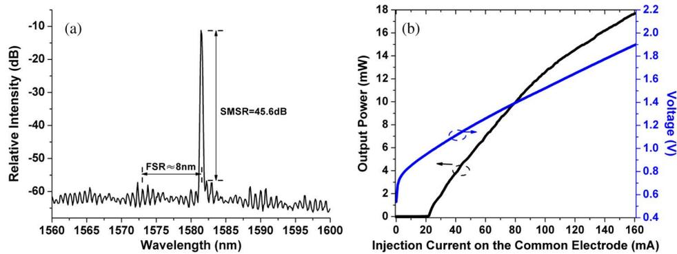
Fig. 2. (a) Single mode emission spectrum of a rectangular ring-FP laser with 45.6 dB SMSR. (b) LIV curve when  $I_r = 61.9$  mA,  $I_t = 79$  mA.
