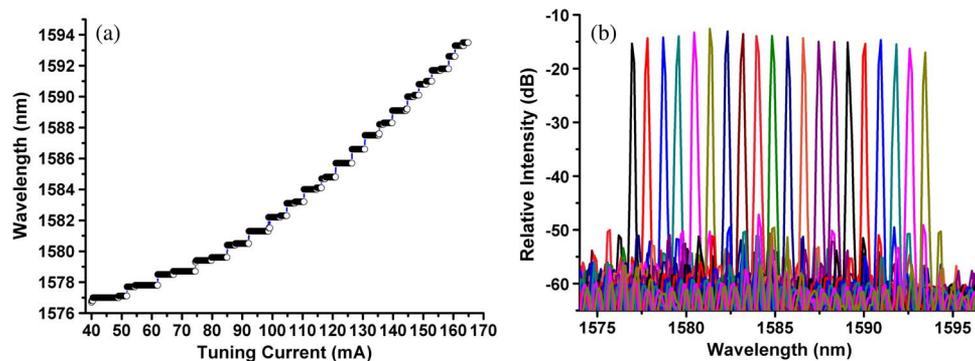
Fig. 3. (a) Measured single-electrode-controlled tuning curve and (b) corresponded superimposed spectra of the 20-channel switching.
