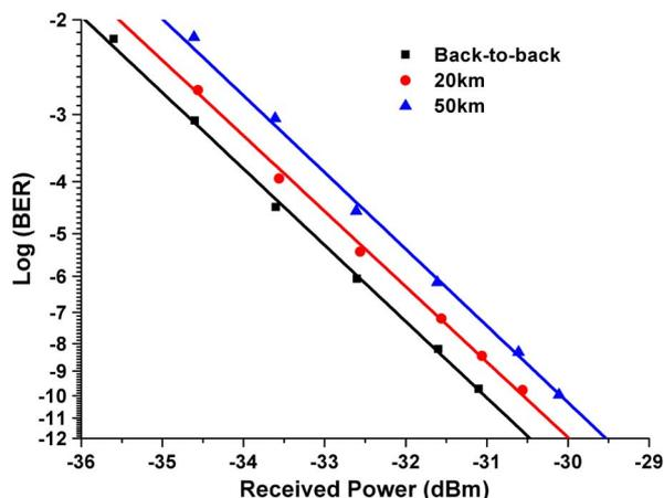
Fig. 7. Measured BER versus received power.
