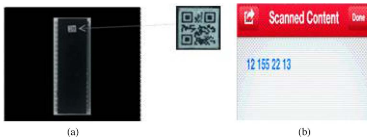
Fig. 4. (a) QR code encoded with a random phase mask placed on an IC and (b) scanned QR code shown in (a).
