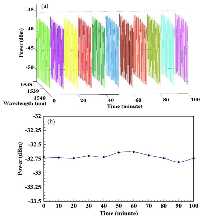
Fig. 7. (a) The MFRL stability under 100 minutes time frame and (b) the average peak power of spectrum line recorded every 10 minutes.
