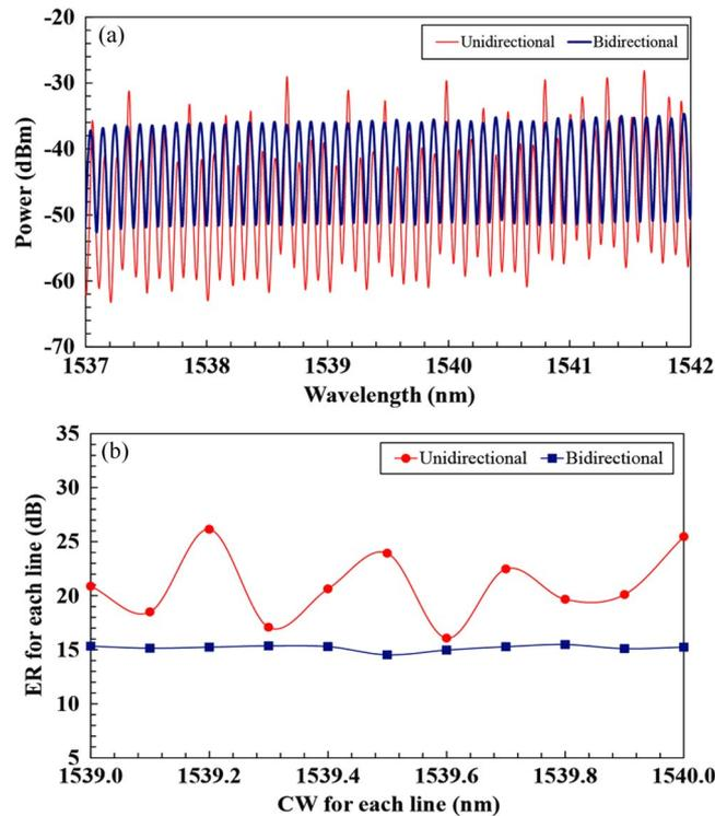
Fig. 4. (a) The MFRL spectrum comparison between unidirectional and bidirectional configuration. (b) ER against CW for each line at different configurations at 1 nm span.
