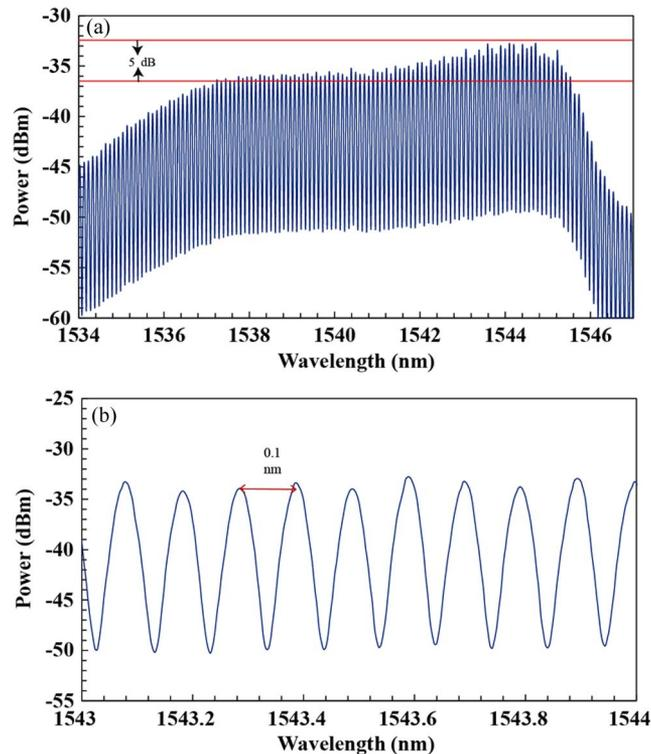
Fig. 2. The flat MFRL spectrum at 350 mA. (b) Magnified view of the spectrum from 1543 to 1544 nm.
