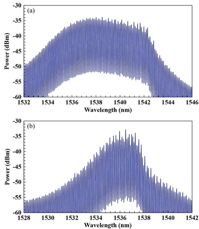
Fig. 5. The spectrum of MFRL when the current is reduced to (a) 250 mA and (b) 150 mA.
