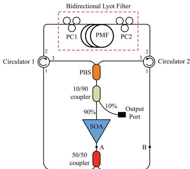
Fig. 1. Experimental configuration of the MFRL generation based on an advanced mechanism of bidirectional Lyot filter.
