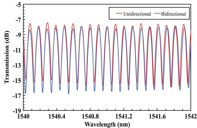
Fig. 3. The measured transmission spectra of unidirectional and bidirectional of Lyot filter.
