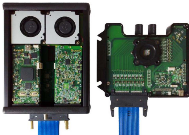
Fig. 11. Picture of the complete TCSPC acquisition system: it includes the photon detection head and the 32-channel module for TCSPC measurements.
