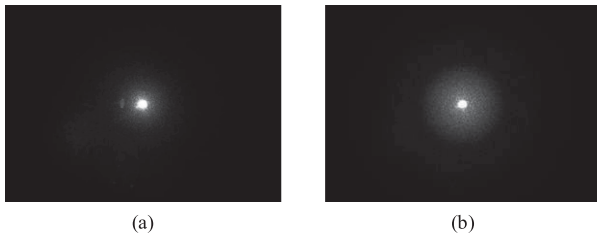
Fig. 10. Comparison of forward scattered light before and after bubble formation: (a) pre-bubble and (b) post-bubble.
