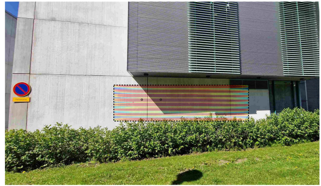
Fig. 3. Photograph of the first test scene: A white partially shaded wall outdoors with the laser illumination pattern illustrated. Two specific measurement spots are marked with circles, which are examined in Fig. 5.
