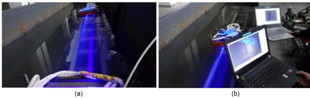
Fig. 6. Underwater experiment. (a) Dynamic range of communication distance measurement. (b) Demonstration of real-time video transmission.
