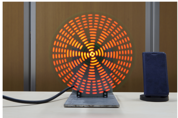
Fig. 10. Test scene where P-Tx shows zone bit-coded light trails.
