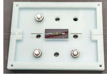
Fig. 6. Photograph of the packaged chip, shown without a removable plastic cover. Note the plastic cover is attached during the measurement while the metal screws securing the white plastic mount in the photo are not present.
