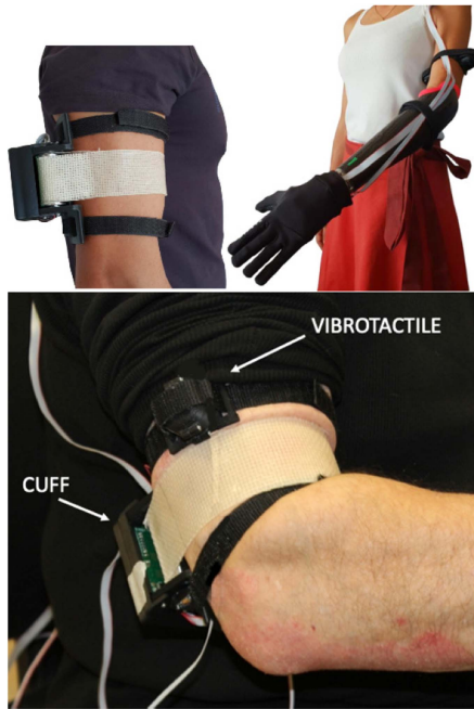
Fig. 1. CUFF, the VibroTactile devices and their combinations applied on the user's arm, during this investigation.
