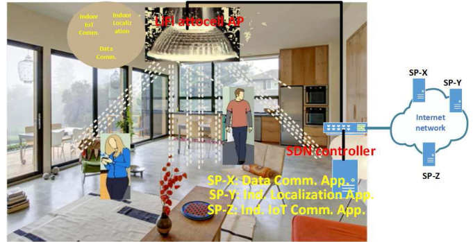
Fig. 1. A use case on indoor LiFi attocell access point slicing.
