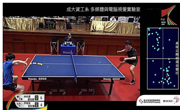
Fig. 8. Snapshot of a table tennis match with real-time ball tracking and the bounce distribution analysis result.
