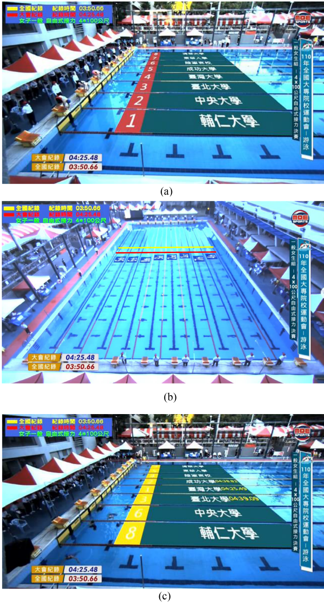
Fig. 11. Three intervals of the AR view of a swimming competition: (a) name list flags before diving, (b) ranking flags during competition, and (c) name list flags of the final ranking.
