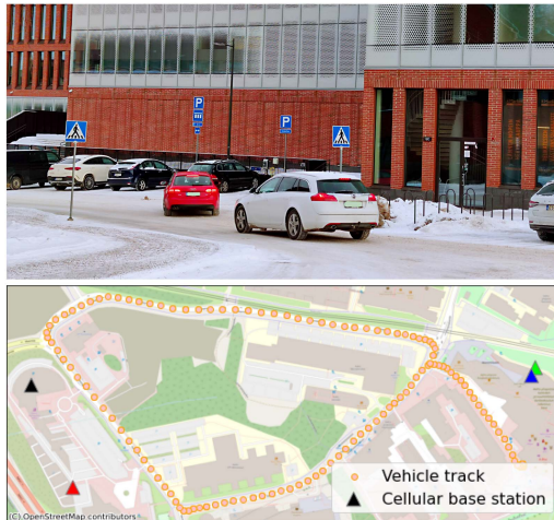
Fig. 4. Measurement setup in Otaniemi, a university campus in Helsinki. The figure shows the white car used for the measurement (on the top) and the test trail (at the bottom).
