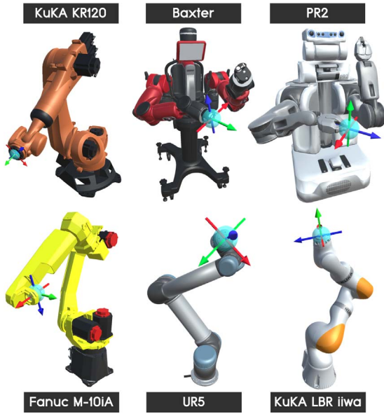
Fig. 8. Robotic arms used for serial inverse kinematics.
