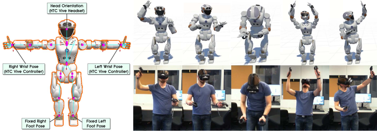
Fig. 18. Motion reconstruction on the NASA Valkyrie robot in virtual reality using the HTC Vive controllers and headset.
