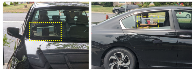
Fig. 10. The two ways in which the radar system was mounted in the moving vehicle for the scenes on the road. In both cases, there was a window in front of the system. For the data from the front facing radar, there are reflections caused by the front of the car, namely the hood and engine.
