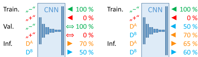
Fig. 4. Illustrating Phase-II (left) and phase-III training (right) using percentage cell viabilities. While phase II splits controls (−, +) between training and validation, phase III trains using all available controls as well as cell viabilities of duplicates inferred in phase II; the latter are exchanged between duplicates D^A and D^B (at the same concentration) of some drug D . Before training, label smoothing is applied (only) to controls; cell viabilities of drug wells are re-used directly. After inference, labels are un-smoothed by normalization in the iTReX web app [40], after which raw cell viabilities 0.80, 0.62, 0.59, 0.56, 0.50 and 0.20 correspond to percentage cell viabilities 100, 70, 65, 60, 50 and 0%, respectively. Colors indicate different groups of wells (green: negative controls; red: positive controls; blue, orange: two duplicates of drug D ), while arrows indicate the way cell viabilities are used (◀: training label backpropagated into the network; ▶: value inferred by the network; ⇔: validation label).
