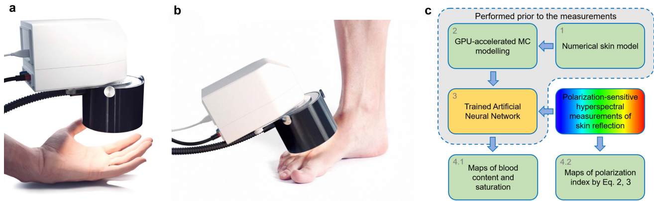
Fig. 2. Presented compact, hand-held hyperspectral imaging system can be easily applied for imaging in an arbitrary selected area of skin. (a) The setup has been verified in measurements of the palmar skin surface. (b) In clinical studies of DM patients, the system has been purposed for measurements in the dorsal surface of feet. (c) Flowchart of data processing. Blocks 1–3 are performed prior to the measurements. Block 4 is performed in line with the data acquisition.
