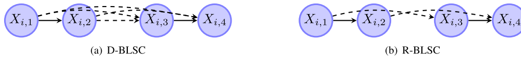
Fig. 5. Two ways of connecting different convolution blocks. (a) Illustrates the dense approach like DenseNet (D-BLSC) where each block in the i -th horizontal line is connected to all the others, (b) illustrates the reduced way (R-BLSC) of connecting blocks from the i -th horizontal line. X_{i,j} represents the convolution block of the cascaded network, where i represents the convolution blocks which are in the i -th horizontal line and j represents the index of the convolution block which is in the i -th horizontal line. X_{i,1} and X_{i,2} represent the encoder block and the decoder block of the first stage network, respectively. X_{i,3} and X_{i,4} represent the encoder block and the decoder block of the second stage network, respectively.
