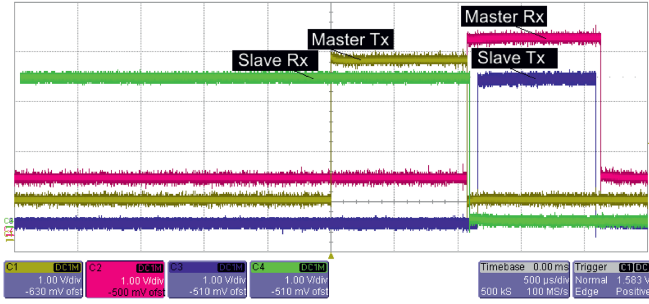
Fig. 3. Oscilloscope screenshots of the GPIO toggling describing, the M/S sending a packet, the M/S complete calibration and the S/M sending a packet back.
