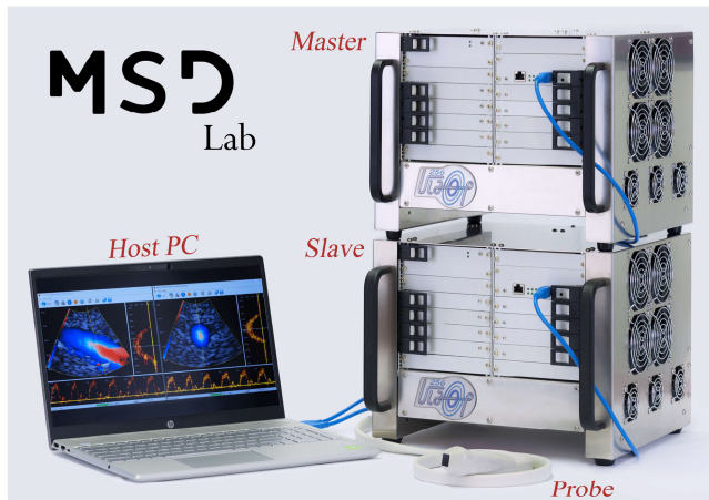
Fig. 3 The 512-channel demonstrator.
