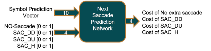
Fig. 9. Inputs and outputs of “Next Saccade Prediction Network” (NSPN).
