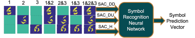
Fig. 6. “Symbol Recognition Neural Network” (SRNN) with one, two and three saccades for a sample of N-MNIST dataset. Each column represents a hyperframe with three frames, each for one saccade direction. When a saccade direction is not available, its frame is left blank.
