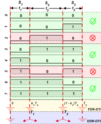
Fig. 2. Possible switching sequences of three consecutive actual voltage vectors.
