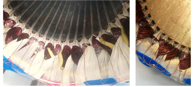
Fig. 5. Extended slot electrodes with a diameter of 0.3 mm (left) and 0.75 mm (right) are installed in a regular 15-kW induction machine.
