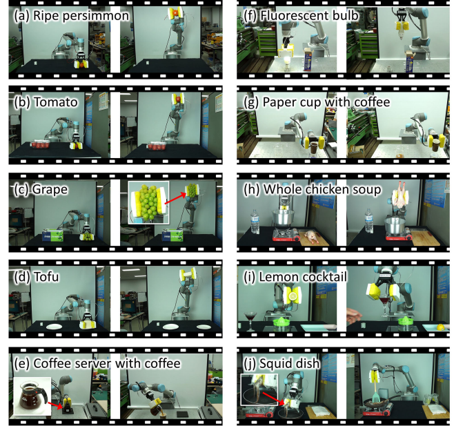
Fig. 16. Examples of practical application of the universal soft gripper. (a) Pick and place of a ripe persimmon. (b) Tomato. (c) Grapes, and (d) tofu (Supplementary video 2). (e) Pouring coffee using a server. (f) Removing a fluorescent bulb from a socket. (g) Pouring coffee out from a paper cup (Supplementary video 3). (h) Cooking whole chicken soup. (i) Making a cocktail with a squeezed lemon. (j) Cooking a squid dish (Supplementary video 4).
