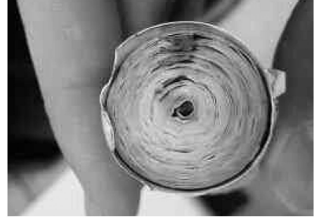
Fig. 2. Sectional photograph of a cylindrical Li-ion cell showing the sandwich structure.
