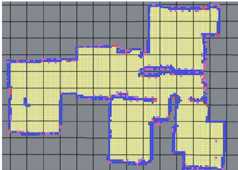
Fig. 12. Generated obstacle grid map for autonomous navigation using the proposed SLAM on NXP4330Q board in a home environment (sequence 3).
