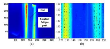
Fig. 9. (a) Raw thermal image at 0.2 s. (b) Thermo optical flow (room in region).
