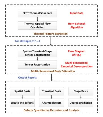
Fig. 6. Flow diagram of the proposed method.
