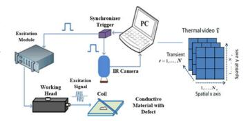
Fig. 3. Inductive thermography diagram.
