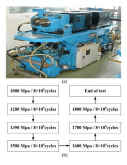
Fig. 8. (a) 160 mm center distance back-to-back contact fatigue test rig facility at Design Unit, Newcastle University, (b) procedure of the stepwise fatigue test ( $8 \times 106$  cycles takes the running for 44.44 h).
