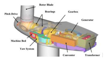
Fig. 1. Configuration of wind turbines.
