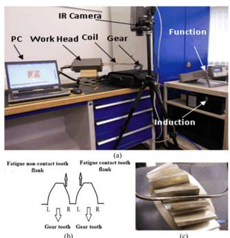
Fig. 7. (a) ECPT experimental system, (b) explanation of gear teeth and the coil placement, and (c) fatigue test gear with inductor coil.
