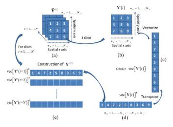
Fig. 5. Illustration of matricizing operation of  $ar{\mathbf{Y}} \imath^{(i)}$ .
