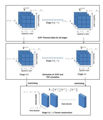
Fig. 4. Flow diagram of spatial-transient-stage tensor construction.
