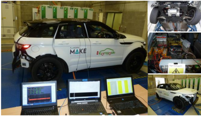
Fig. 3. Range Rover Evoque setup on the rolling road facility at Flanders MAKE (Belgium).
