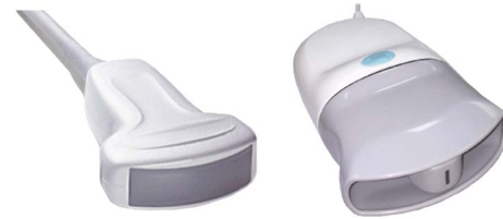
Fig. 1. Comparison of the (left) SonoSite multichannel array transducer [9] and the (right) prototype single-element ultrasound scanner.
