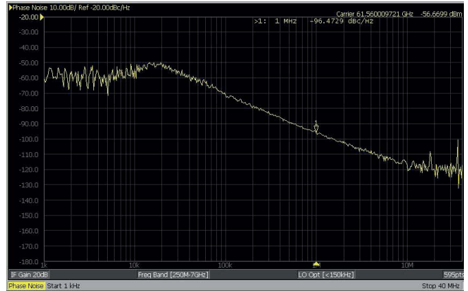
Fig. 34. Measured phase noise at the TX output with f_{LO} = 61.56 GHz.
